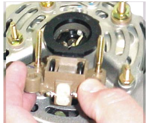
Installing Brush Assembly with Cover Screws and Rubber Seal
